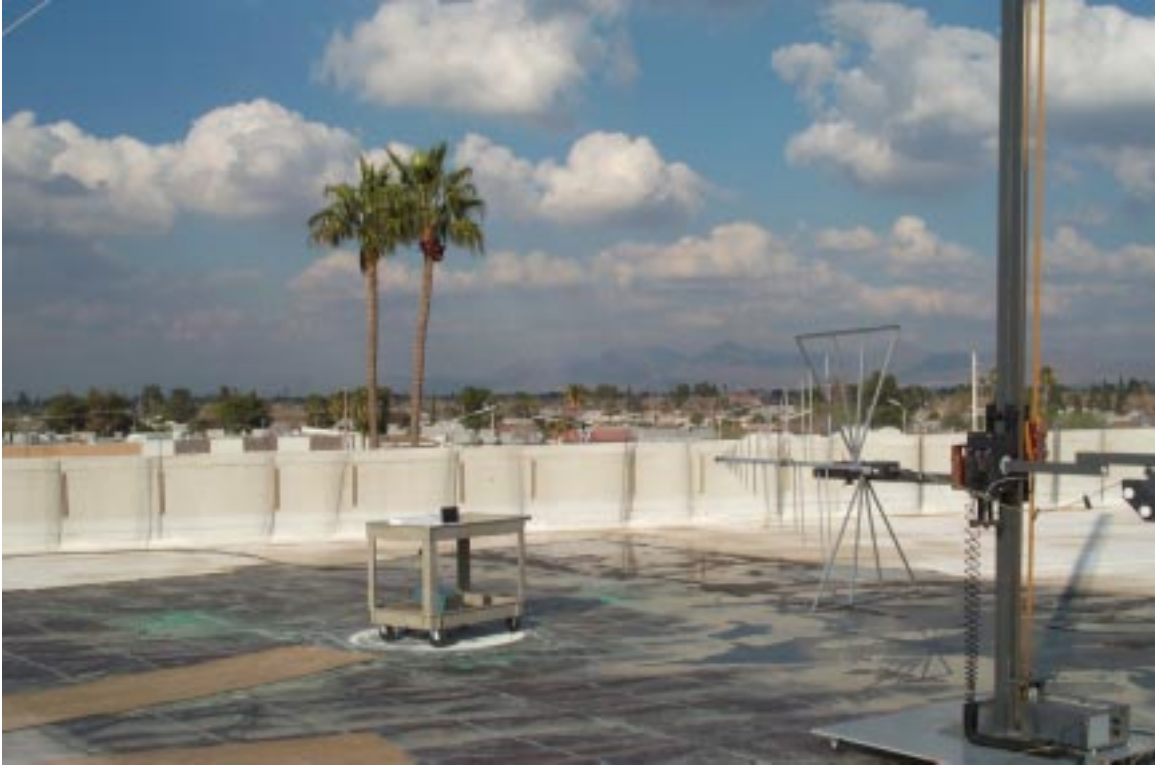
Figure C – 2 Radiated Spurious Emissions Test Setup, OATS
