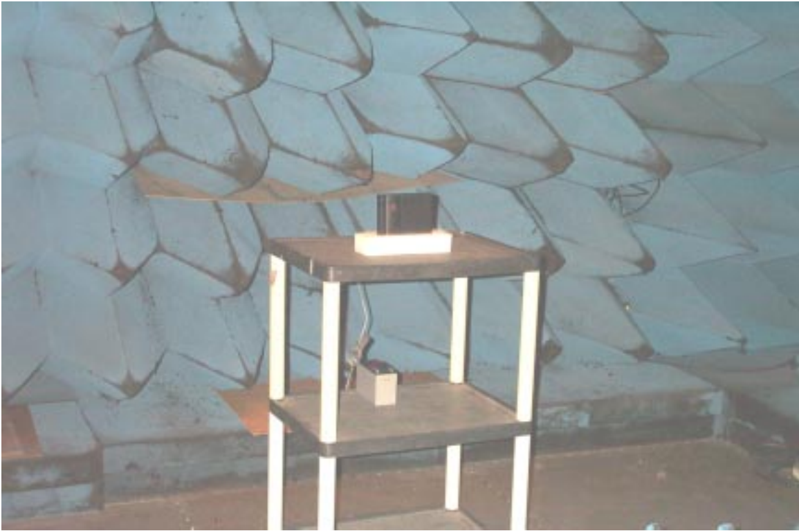
Figure C – 1 Radiated Spurious Emissions Prescan Test Setup, Chamber
