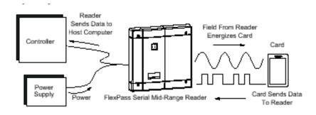
Figure 1 - Serial 610 Smartcard System Diagram
