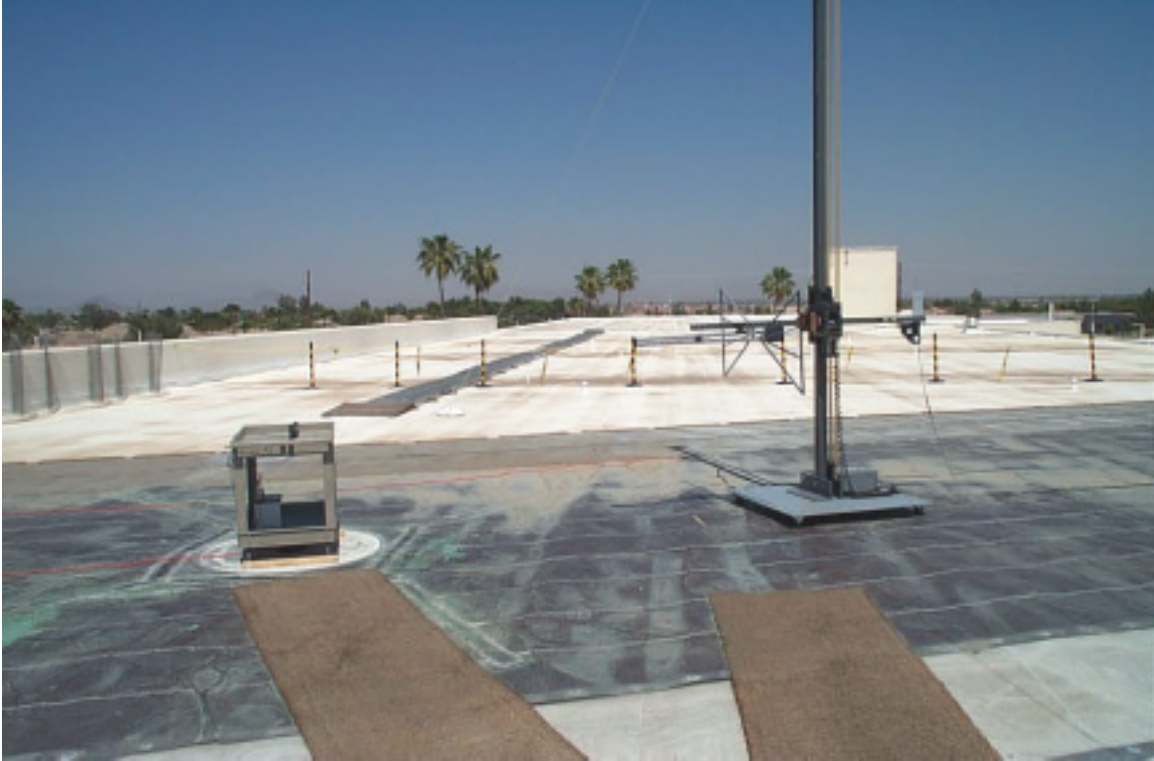
Figure C – 3 Radiated Spurious Emissions Test Setup, OATS
