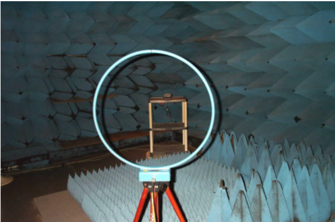
Figure A – 4 Radiated Emissions Test Setup - Loop Antenna
