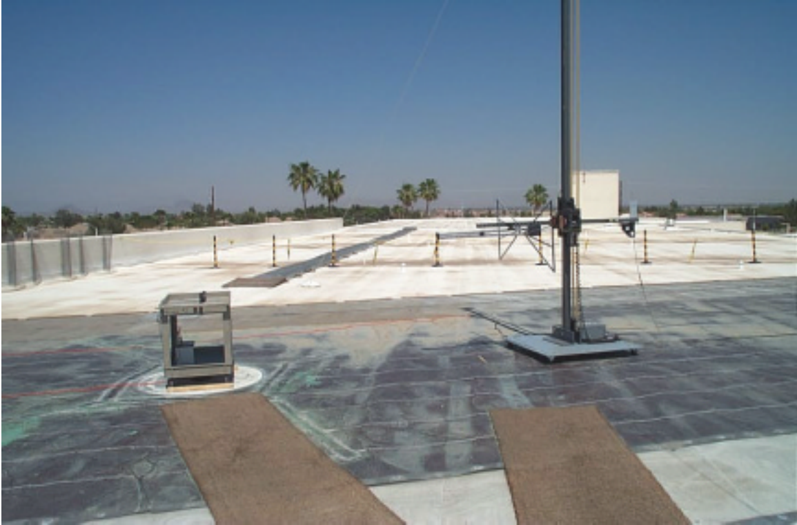
Figure C – 3 Radiated Spurious Emissions Test Setup, OATS
