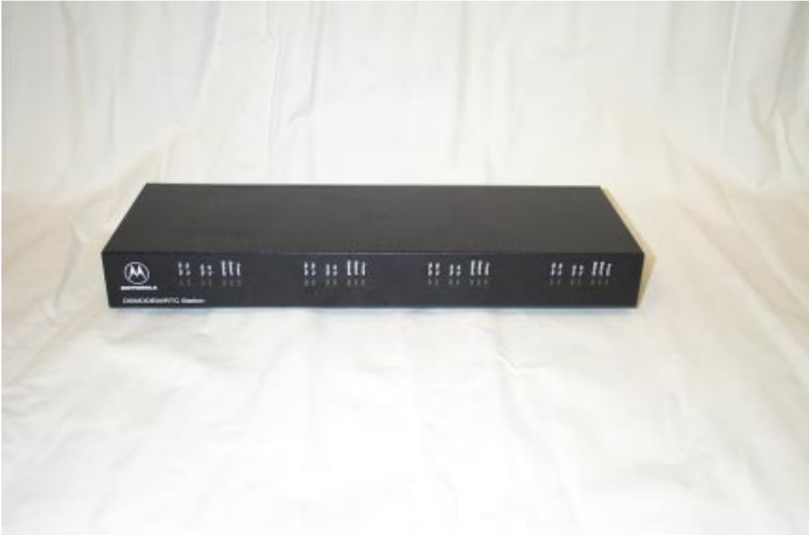
Figure 3.0-1 DSMODEM Base Station External View - Front
