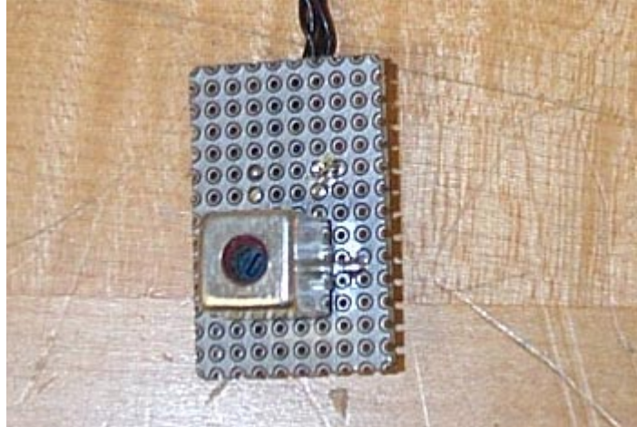
FIGURE 6A - 2 Antenna dummy load
