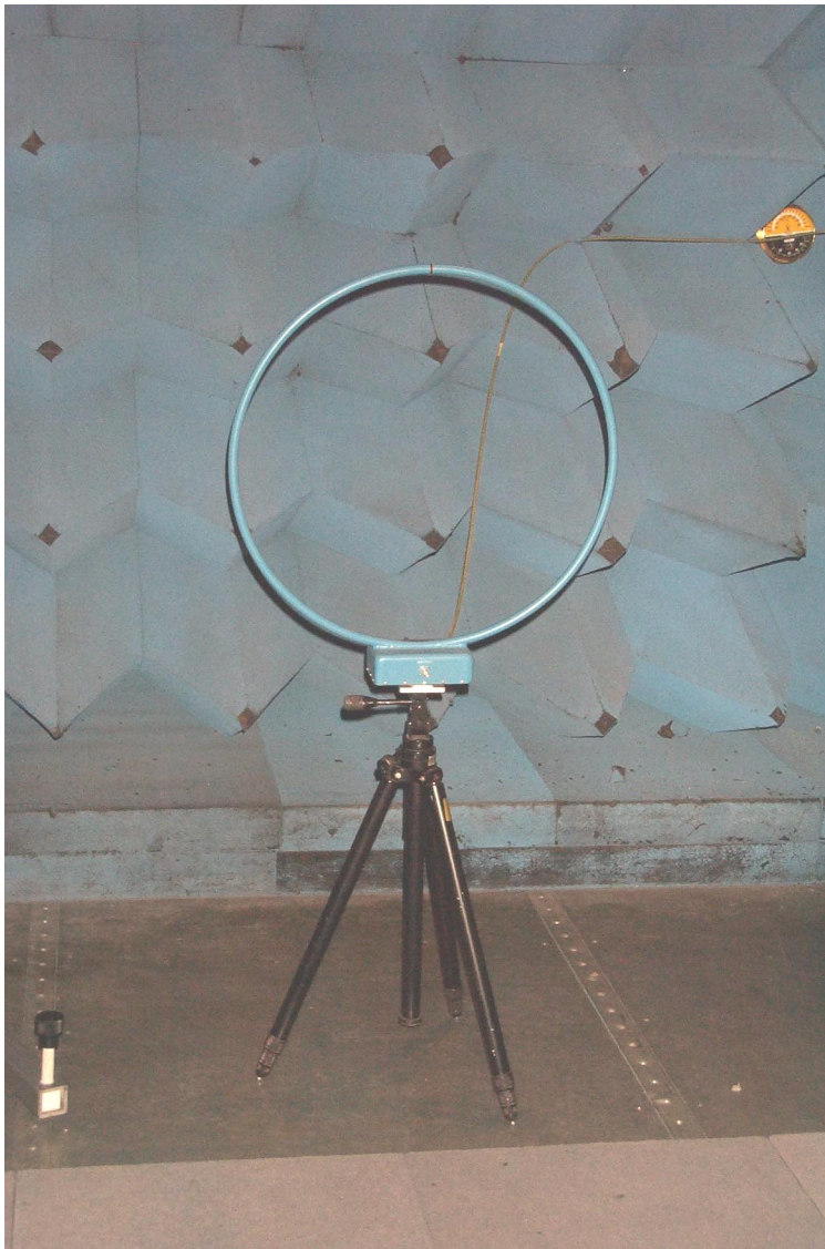
Figure D – 2 Radiated Spurious Emissions – Magnetic Loop
