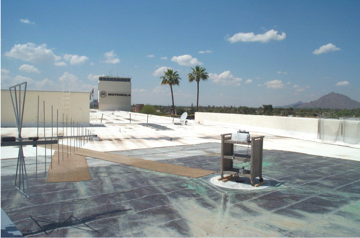
Figure D – 5 Radiated Spurious Emissions Test Setup, OATS
