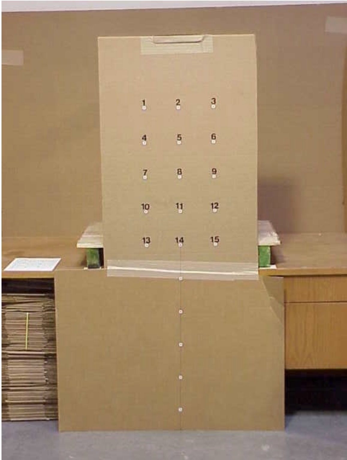
Figure 2. The reader unit was mounted on a wooden platform placed on a wooden desk such that the reader was 79 cm above the floor. A cardboard sheet was used to establish the location of a measurement grid for measurement of electric and magnetic fields.
