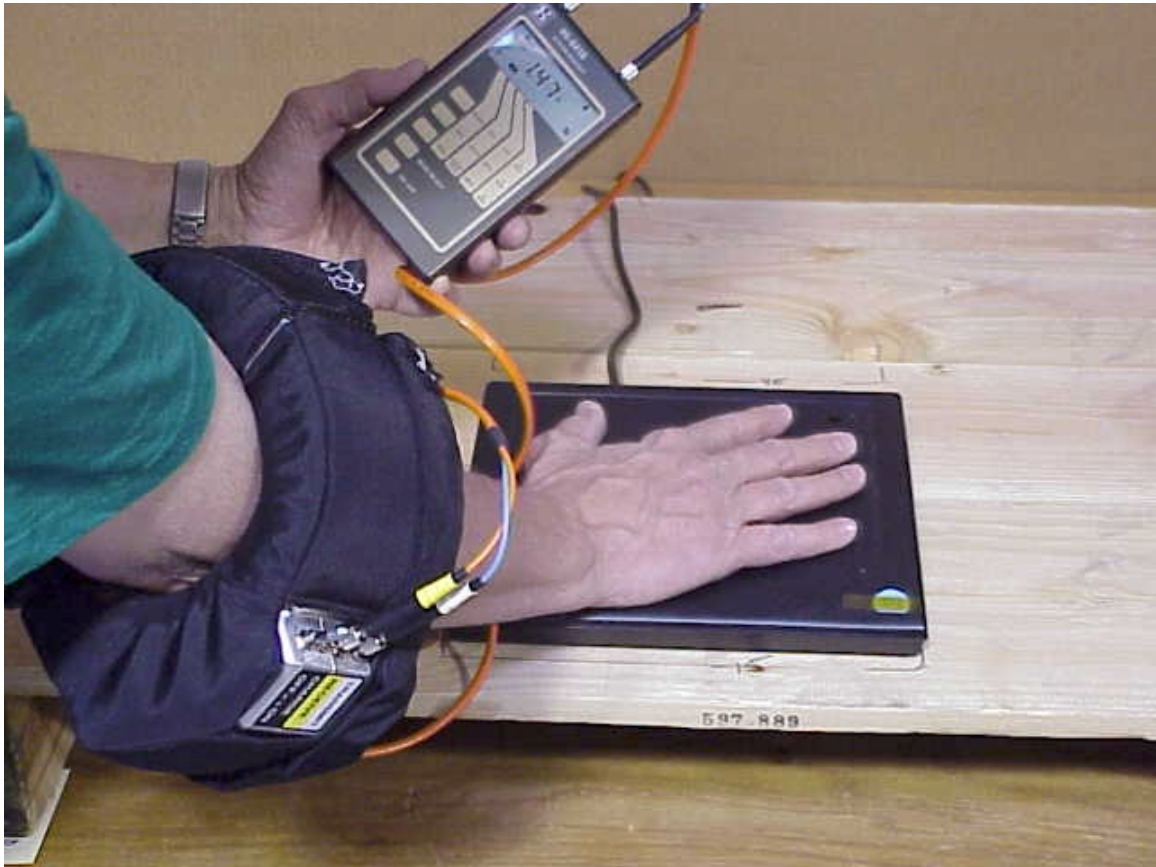
Figure 9. Measurement of contact current was accomplished by placing the RF current transformer around the forearm of the subject and placing the hand in direct contact with the front surface of the reader unit to achieve a maximum indicated current. The subject stood in bare feet for an enhanced electrical connection with the concrete floor.
