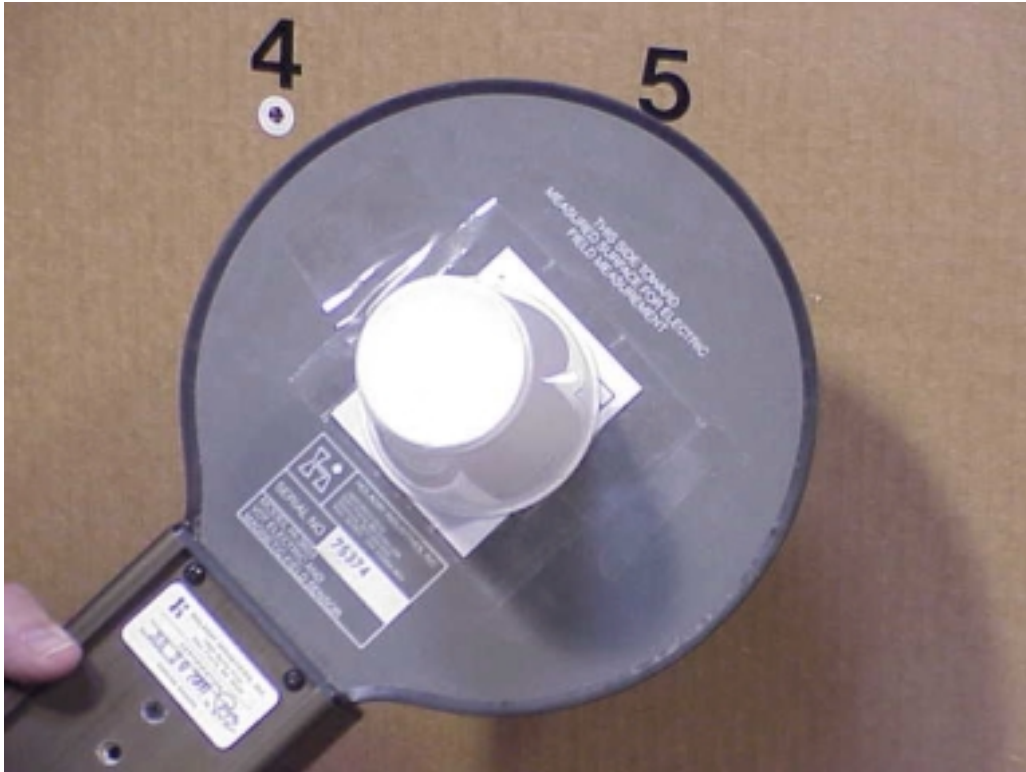
Figure 7. Photograph of the Holaday Industries Model HI-3603 measurement probe showing the attachment of a plastic cup on the sensitive side of the sensor for maintaining a constant measurement distance relative to the cardboard measurement plane.
