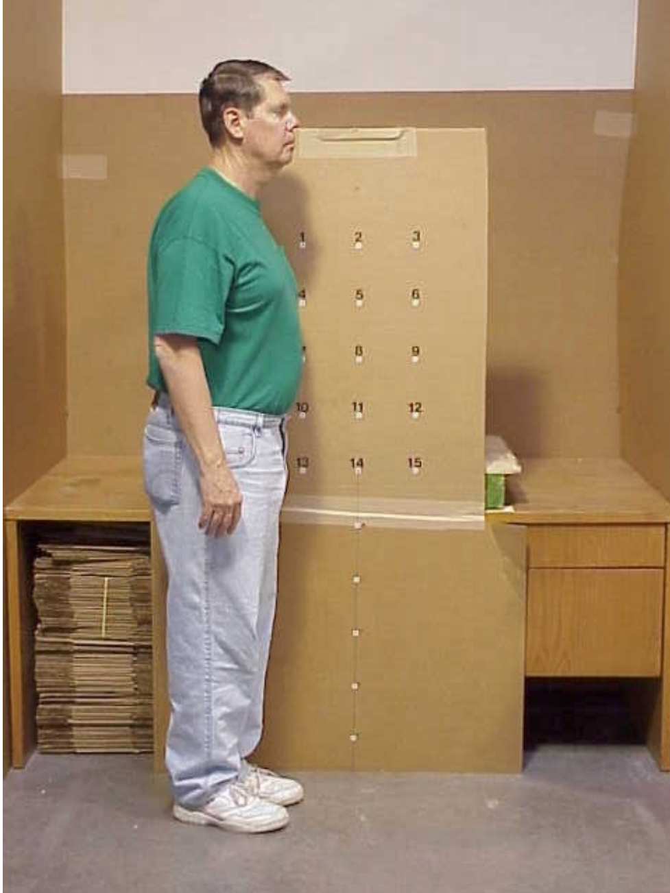
Figure 6. Illustration of the placement of the measurement grid relative to the author standing perpendicular to the cardboard sheet.
