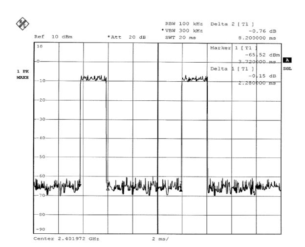
$$20\log(\text{Duty cycle}) = 20\log \frac{2.28 \text{ ms}}{8.2 \text{ ms}} = -11.12 \text{dB}$$
