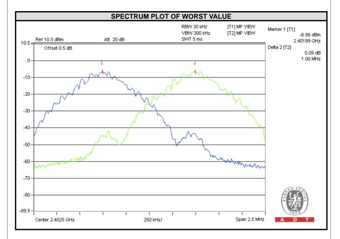
**NOTE:** The minimum limit is two-third 20dB bandwidth. Test results please refer to following graph.
