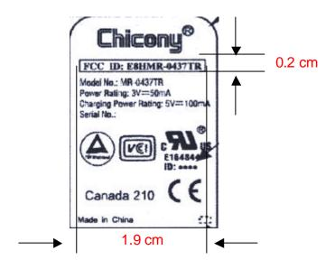
The remained portion of label statement required by FCC is attached in the user's manual.
