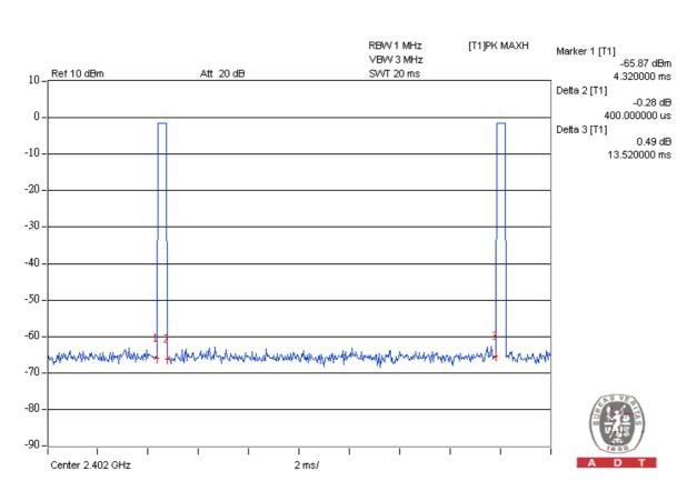
$$20\log(\text{Duty cycle}) = 20\log\frac{0.4 \text{ ms}}{13.52 \text{ ms}} = -30.58 \text{dB}$$
