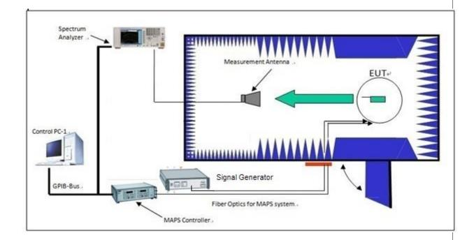
Figure 1. 2D antenna pattern test system.
