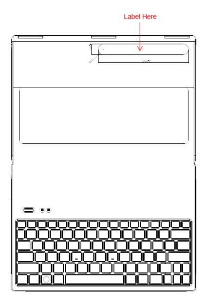
The IC Label will be placed on the equipment as shown in the photograph below.
