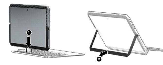
NOTE: If you close the kickstand, you can leave the keyboard attached and rotate the keyboard so that the back of the keyboard rests against the back of the behind the tablet. The keyboard keys and TouchPad are locked to prevent you from accidently typing while the keyboard is in this position.
