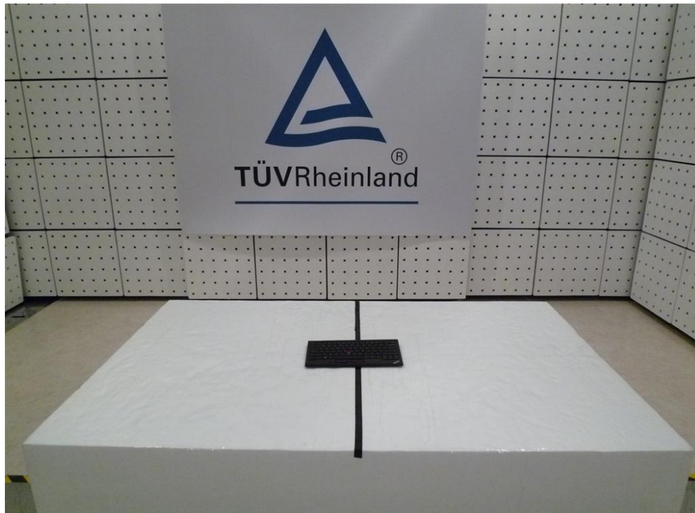
Photograph 2: Set-up for Spurious Emissions (Back View 1)
