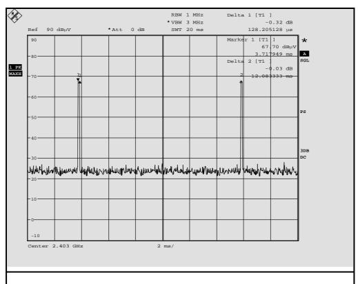
$20 \log (Duty cycle) = 20 \log (0.128 \text{ ms} / 12.08 \text{ ms}) = -39.5 \text{ dB}$
