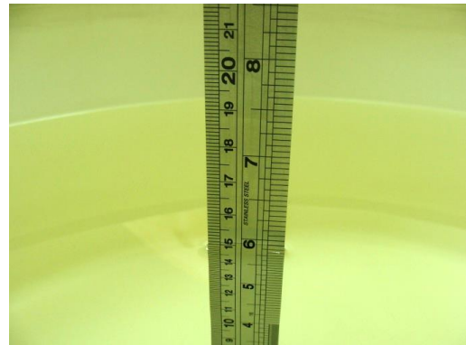
Fig 6.2 Photo of Liquid Height for Body SAR
