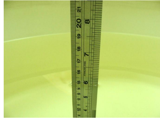
Fig 6.2 Photo of Liquid Height for Body SAR
