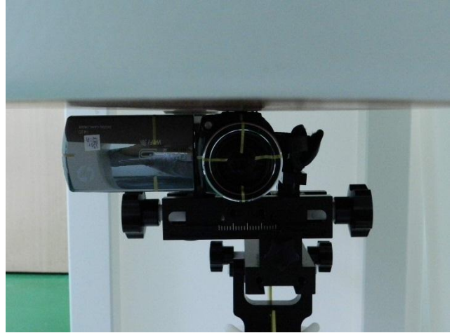
Back of the DUT with Phantom 0 cm Gap (Display screen open up to 90 degrees)
