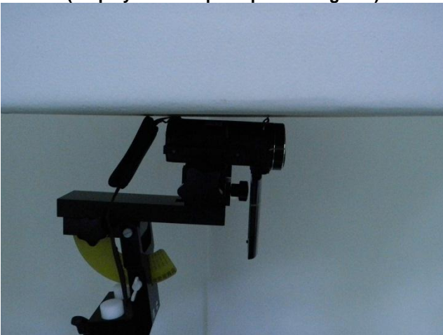
Right Side of the DUT with Phantom 0 cm Gap (Display screen open up to 90 degrees)
