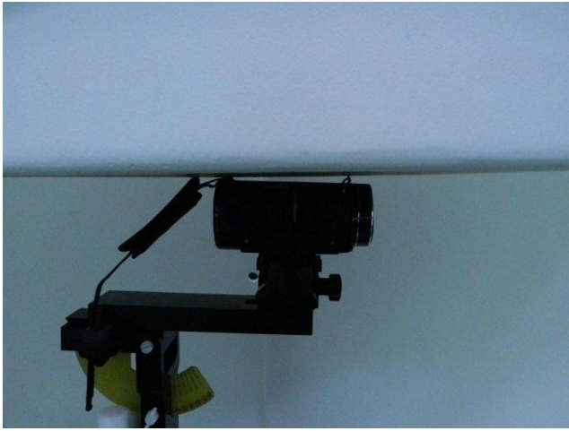
Right Side of the DUT with Phantom 0 cm Gap (Display screen folded up)
