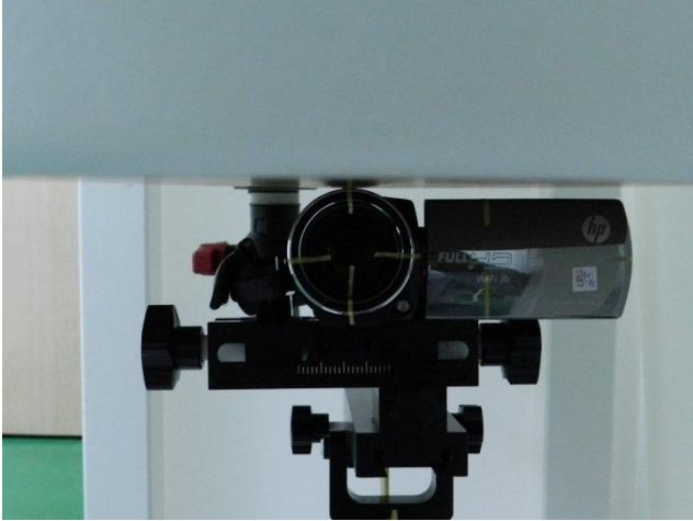
Front of the DUT with Phantom 0 cm Gap (Display screen open up to 90 degrees)
