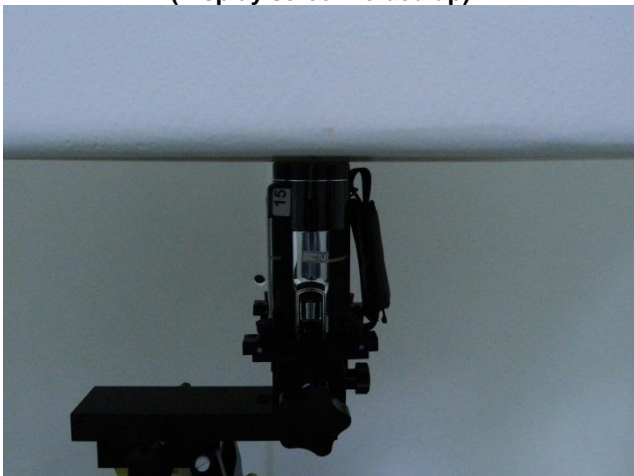
Top Side of the DUT with Phantom 0 cm Gap (Display screen folded up)
