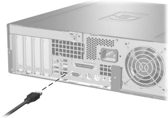
Connecting the USB Cable to the Computer
