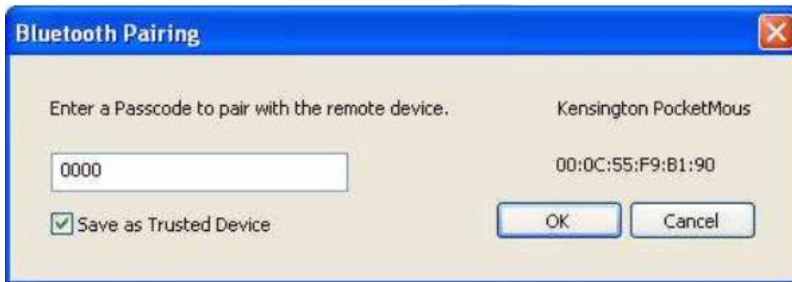
Figure 4-2. Entering Bluetooth Pairing Passcode
