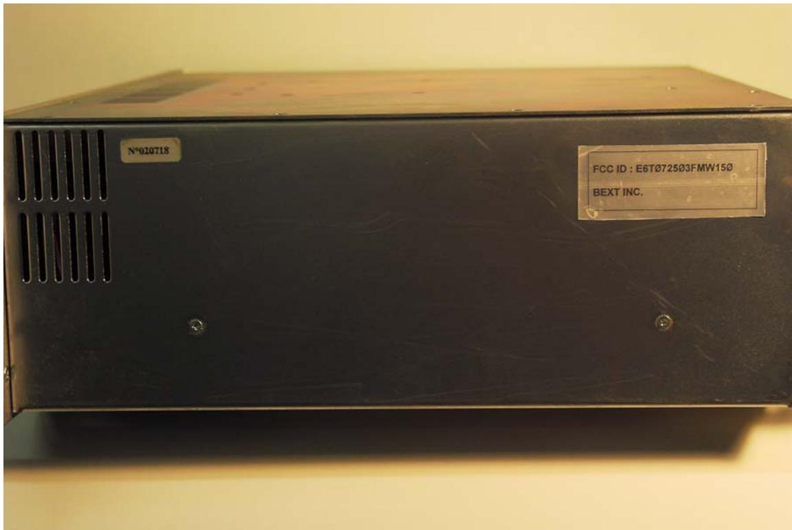
The FCC ID Label is located on the right side of the XT 150 transmitter unit while facing the front panel of the transmitter unit.
