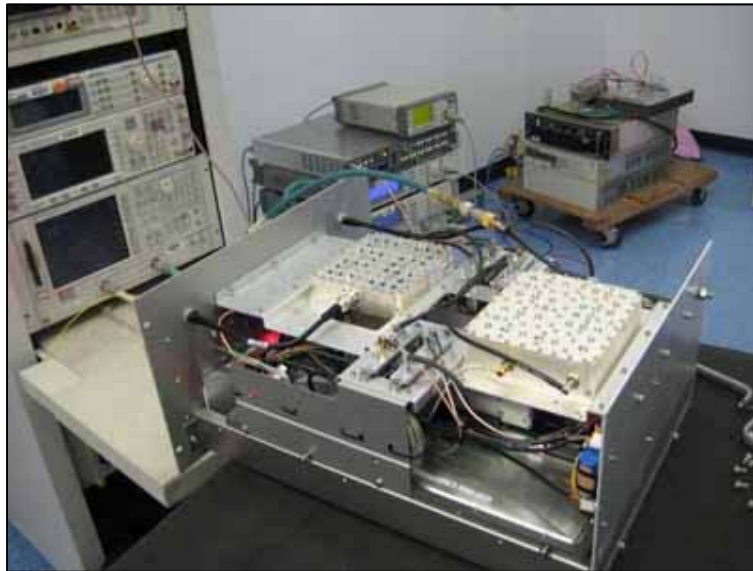
AMPLIFIER GAIN AND BANDWIDTH TEST SET UP
