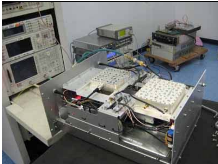
OUT OF BAND REJECTION TEST SET UP
