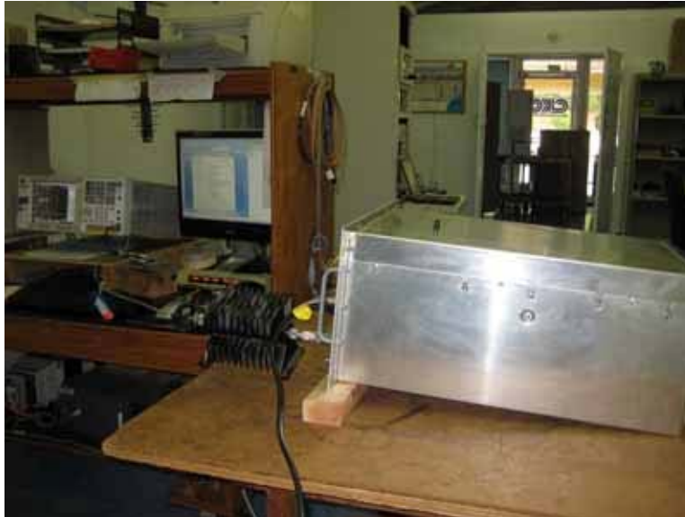
INTERMODULATION TEST SET UP
