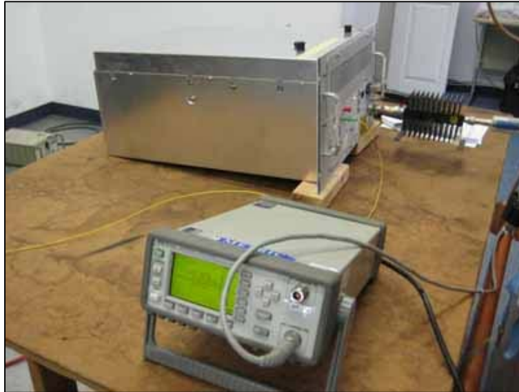
RF OUTPUT POWER TEST SET UP
