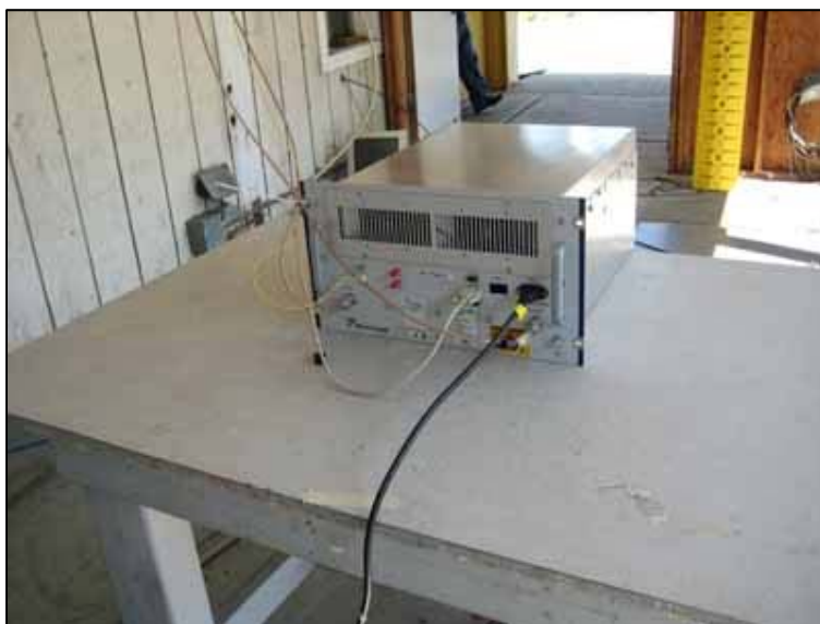
2.1053 RADIATED SPURIOUS EMISSIONS TEST SET UP
