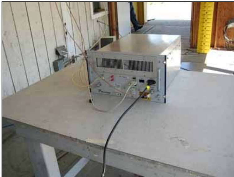
2.1053 RADIATED SPURIOUS EMISSIONS TEST SET UP
