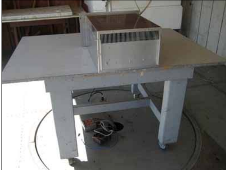
2.1053 RADIATED SPURIOUS EMISSIONS TEST SET UP
