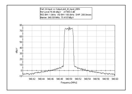
FCC PART 24 OUTPUT PLOT - MIDDLE CHANNEL IDEN
