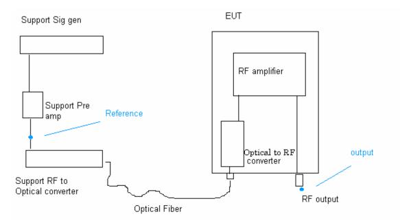
Measured gain = Output - Reference (dB)
