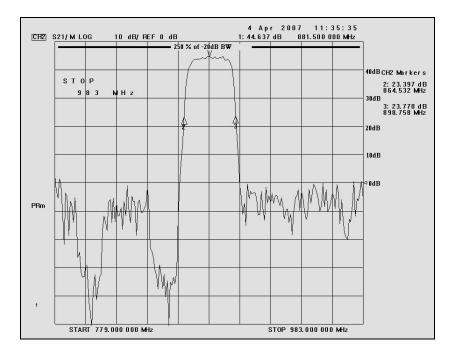
The gain-versus-frequency response of the amplifier from the mid band Fo of the pass band up to at least fo + - 250% of the 20dB Bandwidth.
