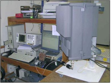
**Test Conditions:** The EUT is a RF amplifier. The manufacturer does not provide an antenna for sale with the product, hence EIRP is not measured nor calculated. The RF power of the EUT was measured at the antenna port in accordance with **RSS 131, 4.3.1** requirement.
