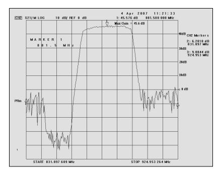
The internal control is adjusted to the nominal gain for which equipment certification is sought. Maximum measured gain = 45.6 dB
