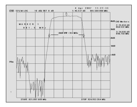
With the aid of a Vector Network analyzer, the -20 dB Bandwidth is measured.
