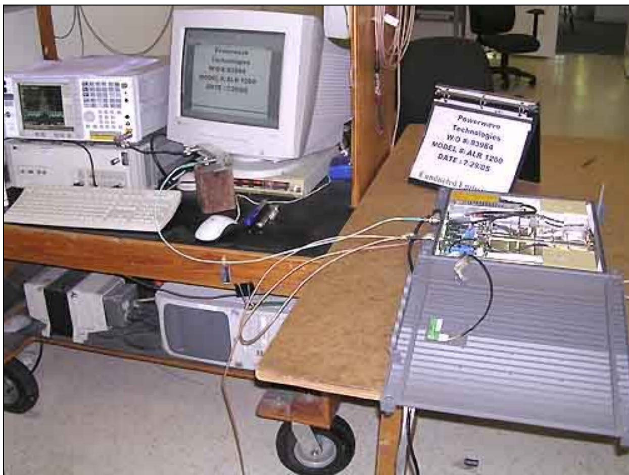
PHOTOGRAPH SHOWING DIRECT CONNECT TEST SETUP
