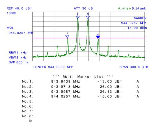
PLOT #: 9 Intermodulation with 3 RF signal inputs/outputs Fc: 944 MHz, Fc - 25.0 kHz & Fc - 50.0 kHz RF Input: (1) -7.8 dBm, (2) -8.3 dBm, (3) -8.5 dBm
