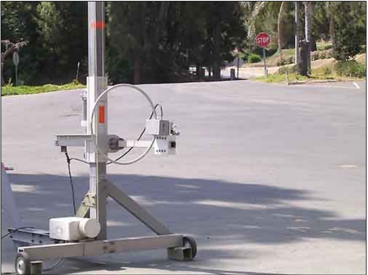
Radiated Emissions - Loop Antenna
