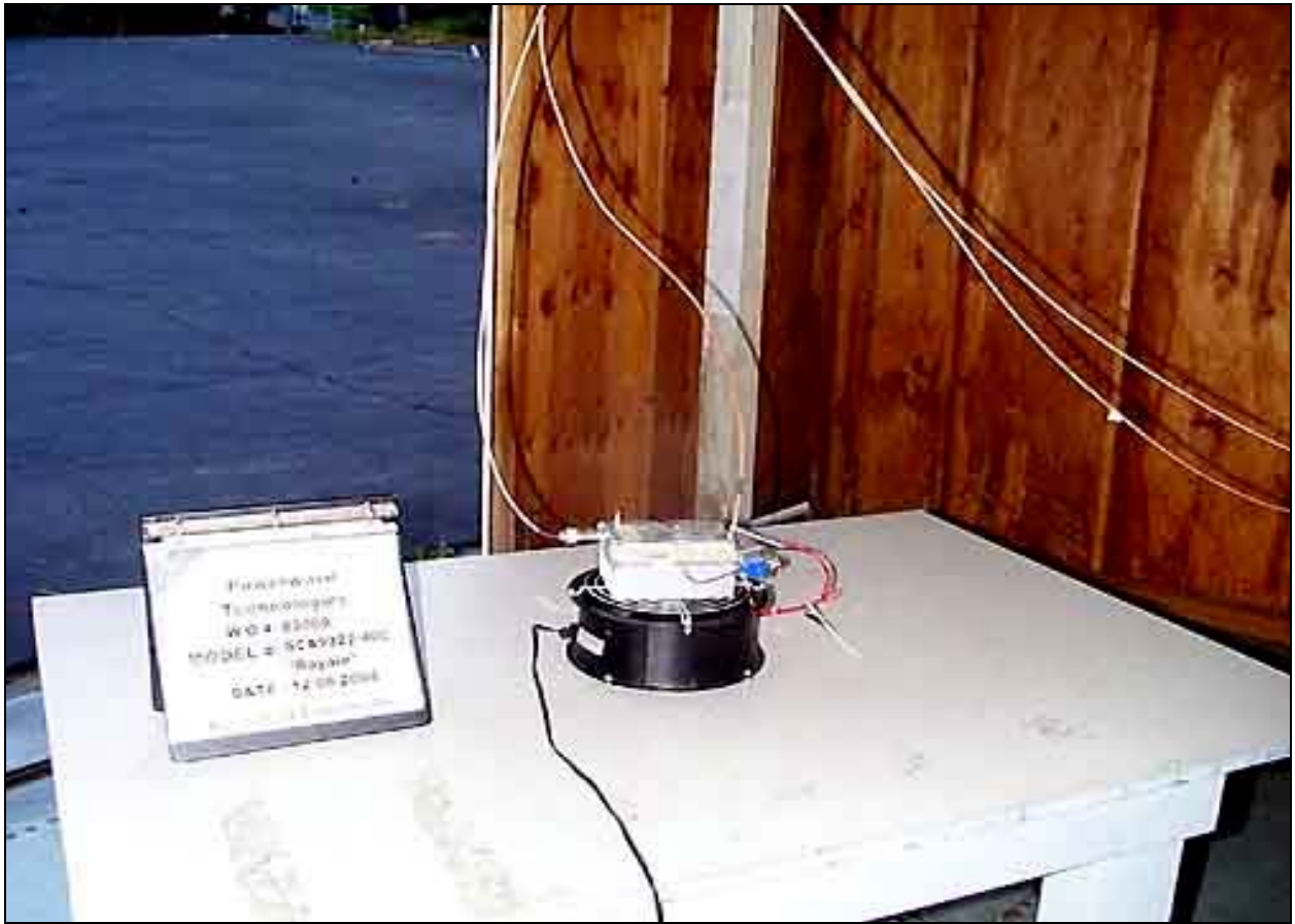
Radiated Emissions - Front View
