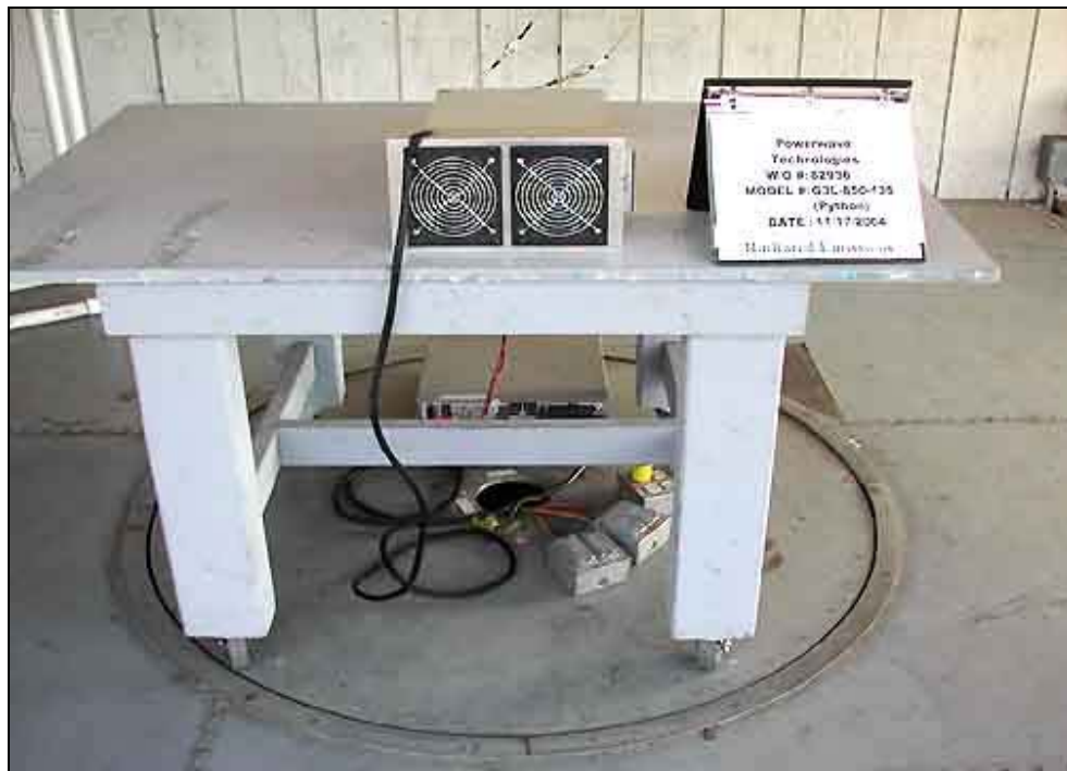
Radiated Emissions - Front View
