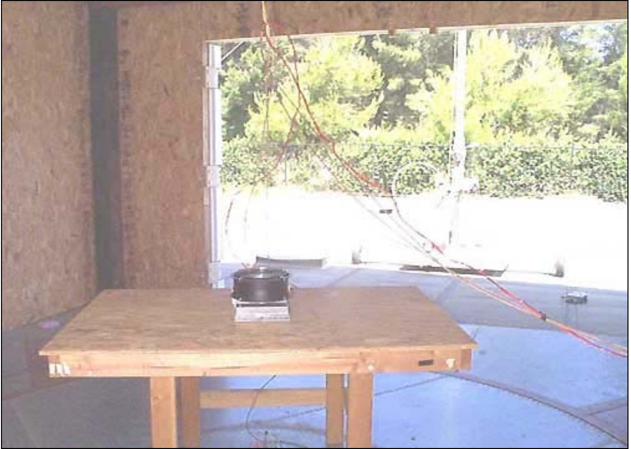
Radiated Emissions - Front View Loop Antenna
