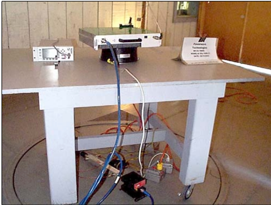
OATS Test Setup - Front View - AC
