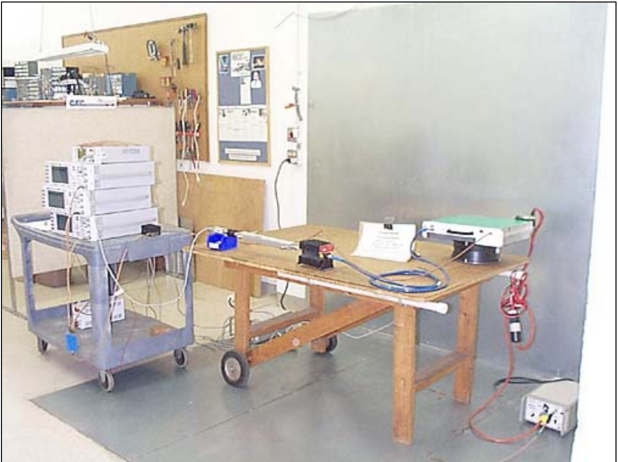
Mains Conducted Emissions - Front View - AC
