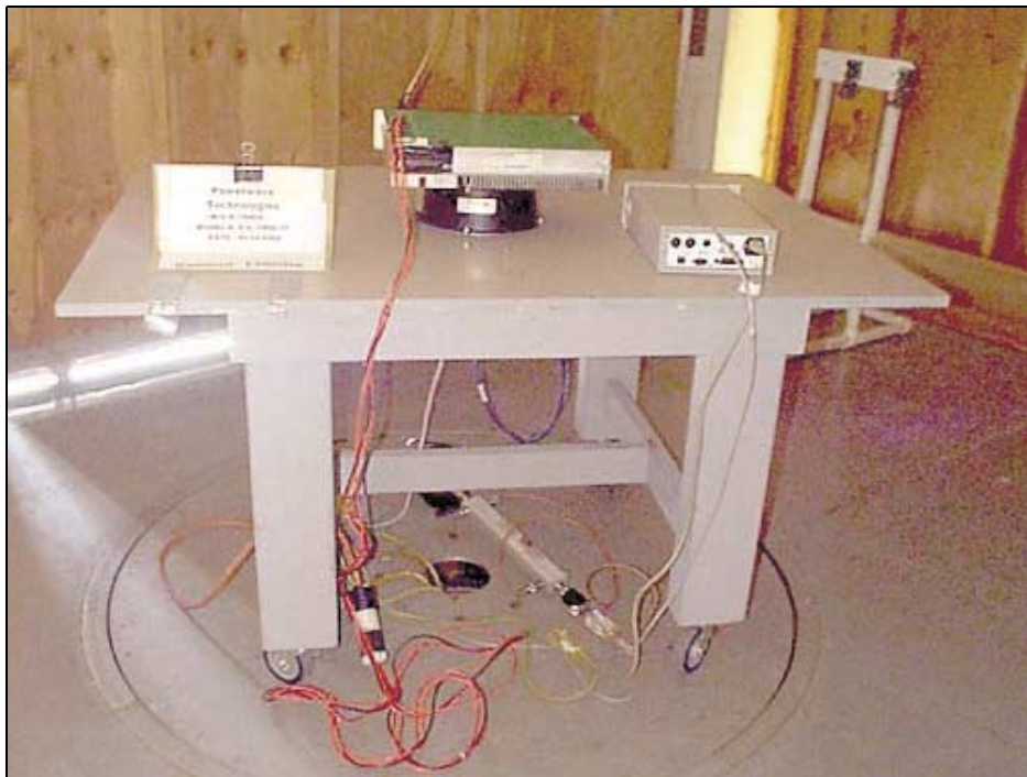
OATS Test Setup - Back View - AC
