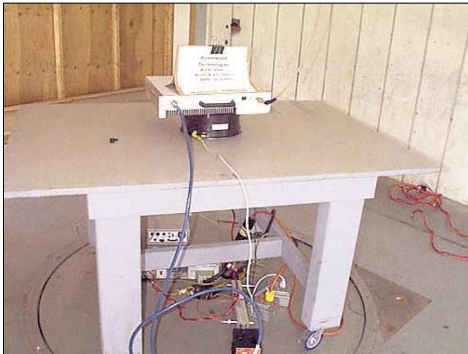
OATS Test Setup - Front View - DC
