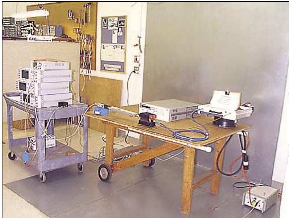
Mains Conducted Emissions - Front View - DC
