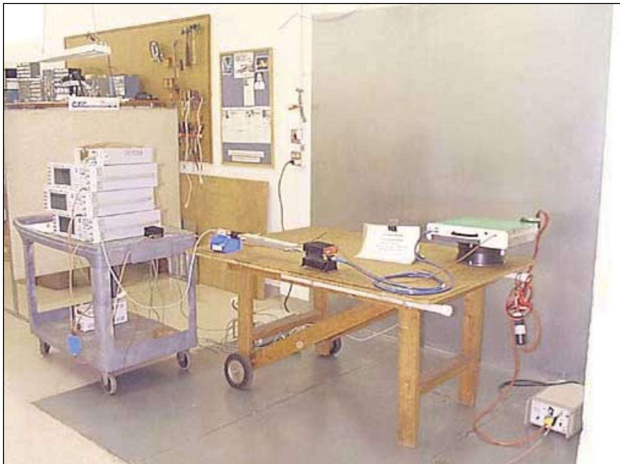
Mains Conducted Emissions - Front View - AC
