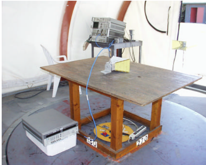
1 - 18 GHz Substitution Method Setup
