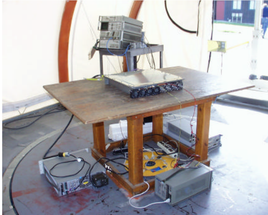
1 – 18 GHz Radiated Emission Setup
