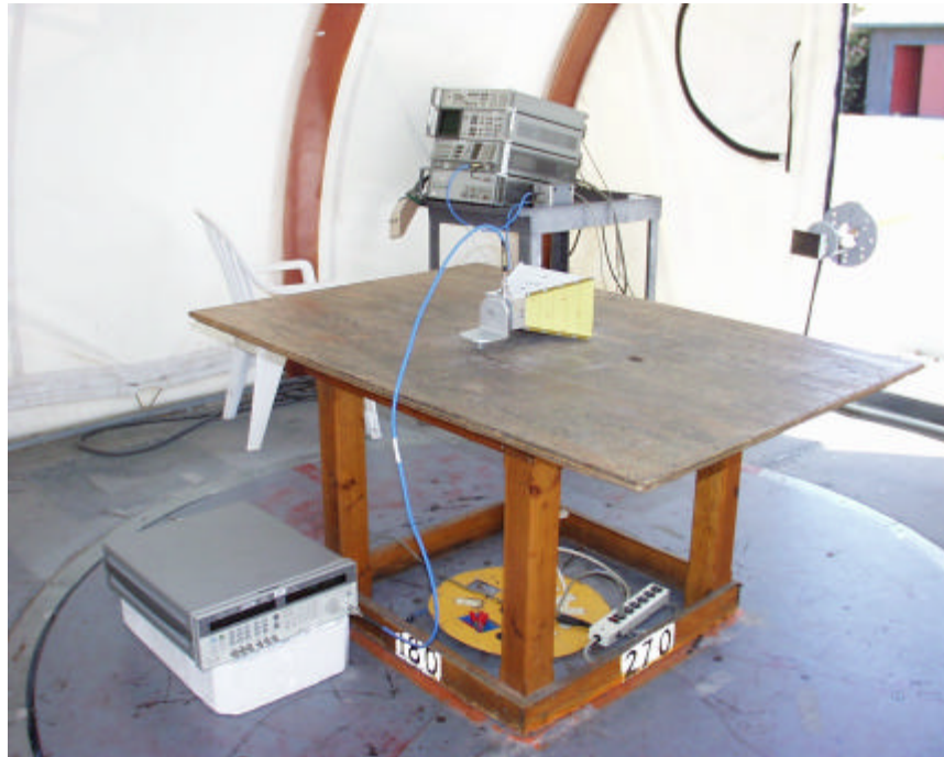
Above 18 GHz Substitution Method Setup
