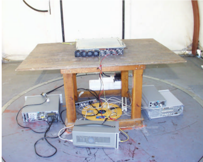
Radiated Emission Setup
