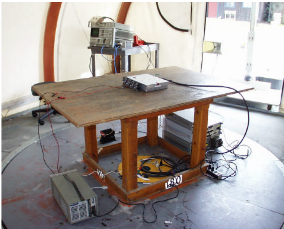
1 - 9GHz Radiated Emission Setup
