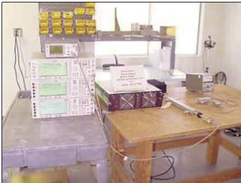
Direct Connect at Antenna Port Test Setup - Front
