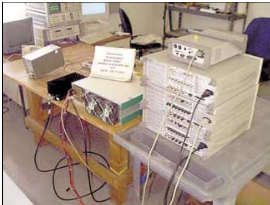
Direct Connect at Antenna Port Test Setup - Back
