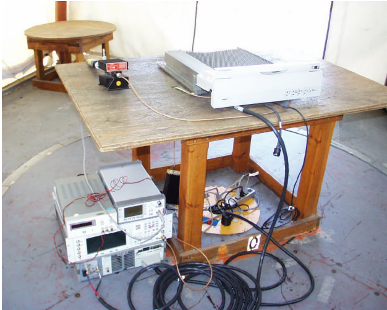
Part15 front view Radiated Emission Setup
