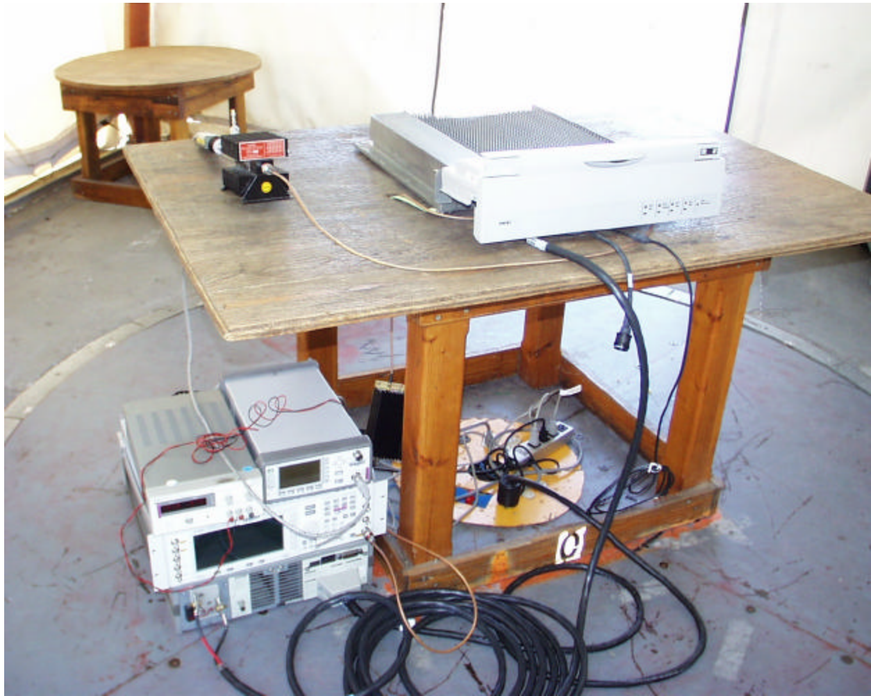
Part15 front view Radiated Emission Setup
