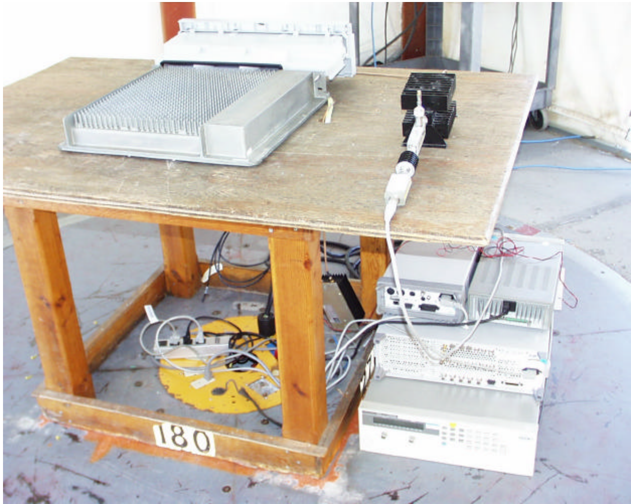
Part15 back view Radiated Emission Setup
