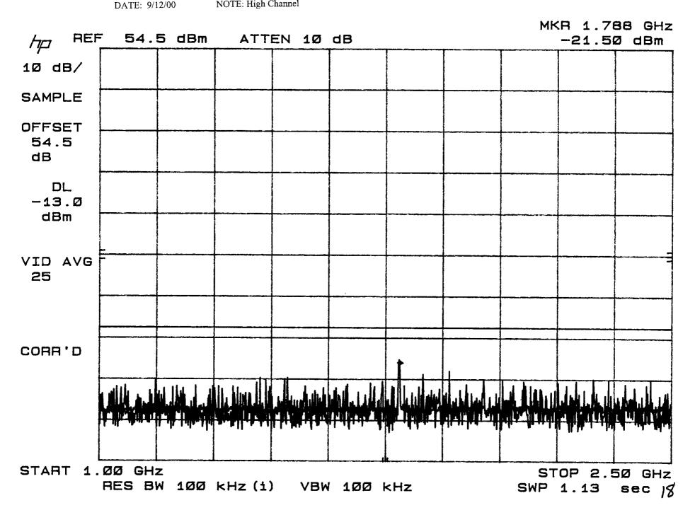
TEST: Conducted Spurious NOTE: High Channel
