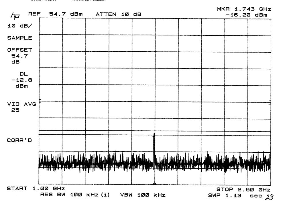
TEST: Conducted Spurious NOTE: Low Channel
