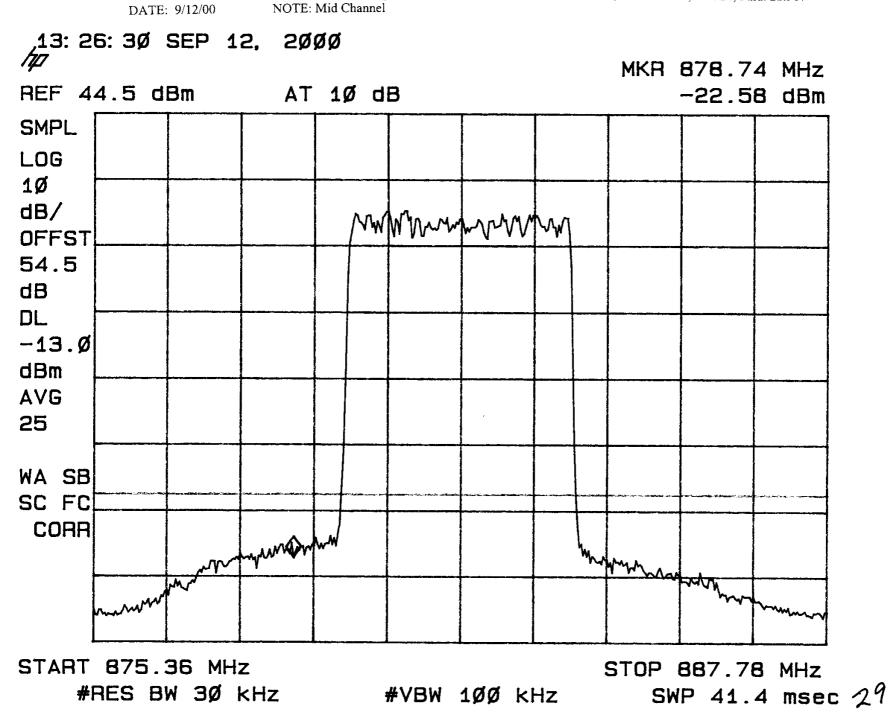
TEST: Conducted Spurious NOTE: Mid Channel
