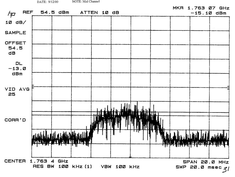
TEST: Conducted Spurious NOTE: Mid Channel
