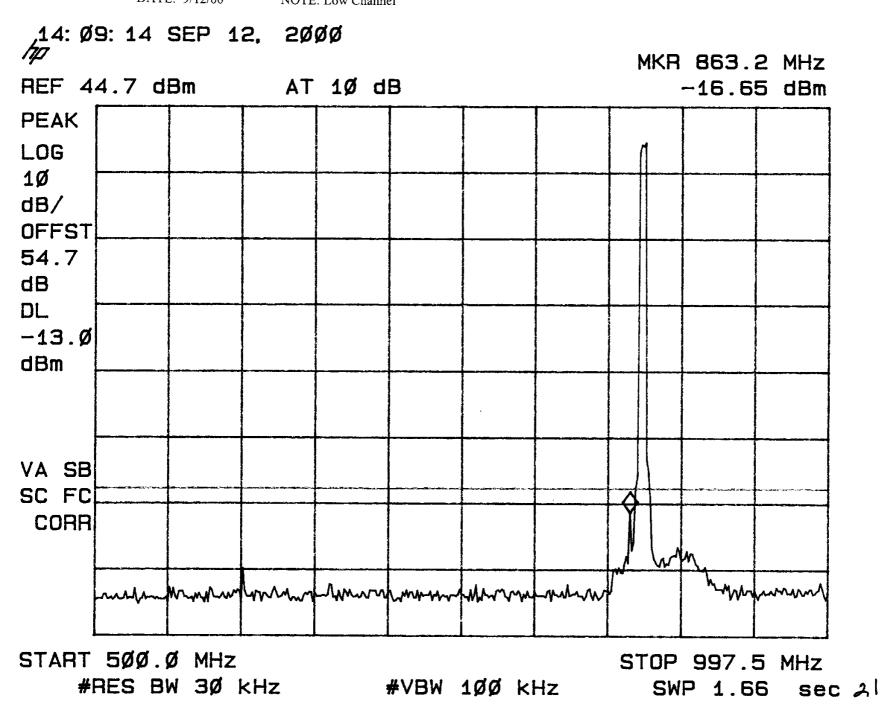
TEST: Conducted Spurious NOTE: Low Channel
