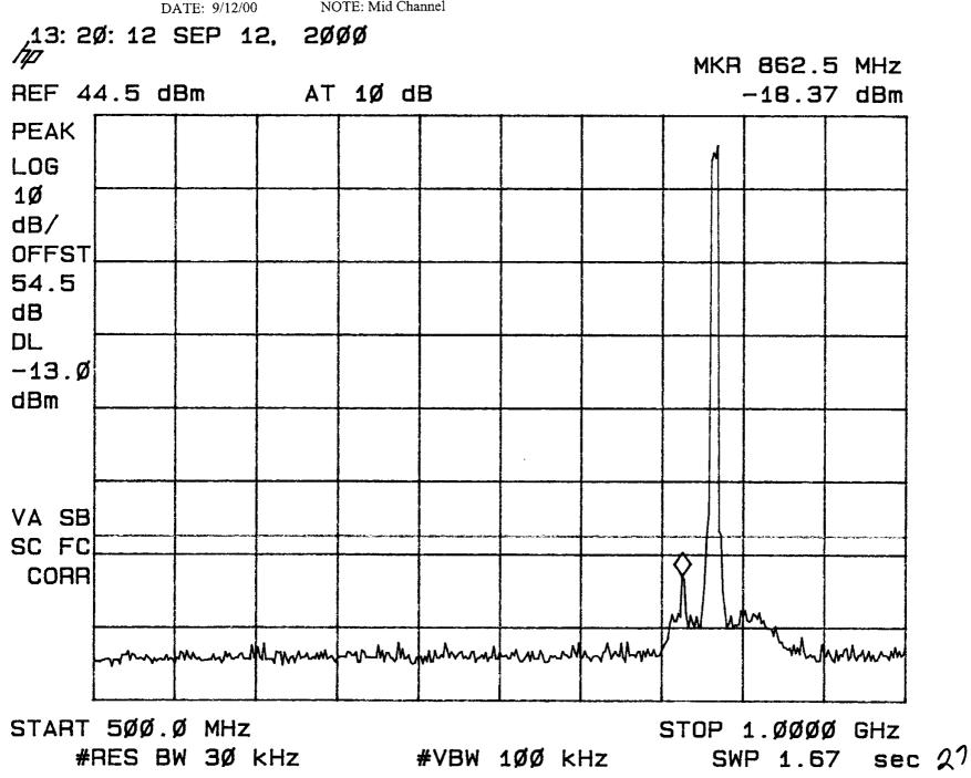
TEST: Conducted Spurious NOTE: Mid Channel
