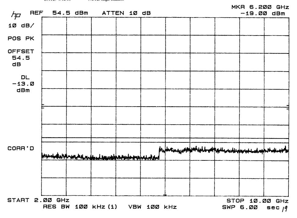
TEST: Conducted Spurious NOTE: Low Channel
