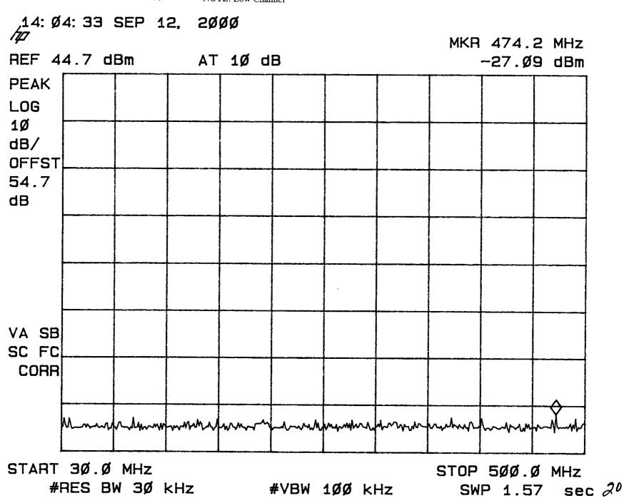
TEST: Conducted Spurious NOTE: Low Channel
