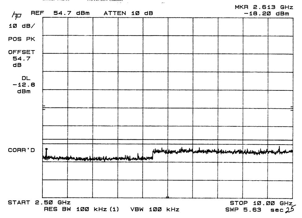
TEST: Conducted Spurious NOTE: Mid Channel
