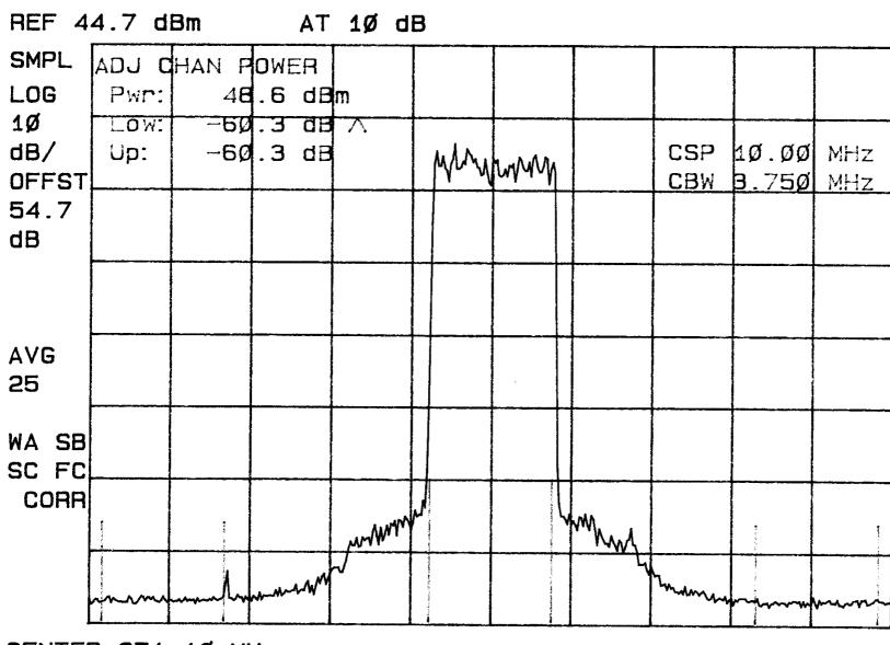
TEST: Adjacent Channel Power NOTE: Mid Channel
