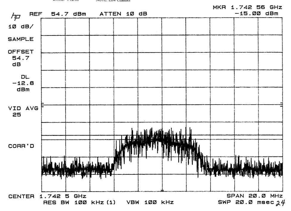
TEST: Conducted Spurious NOTE: Low Channel
