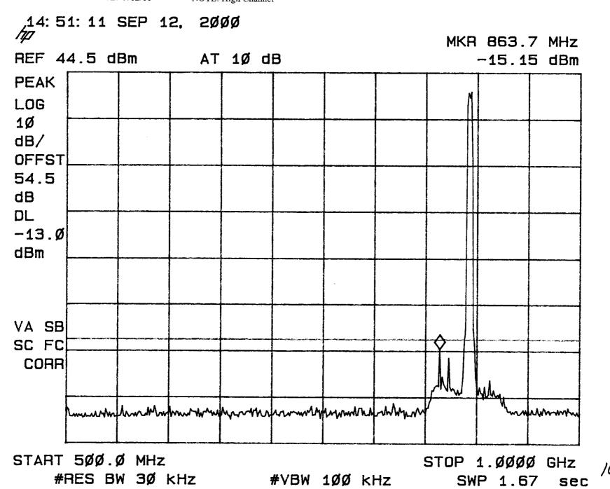
TEST: Conducted Spurious NOTE: High Channel
