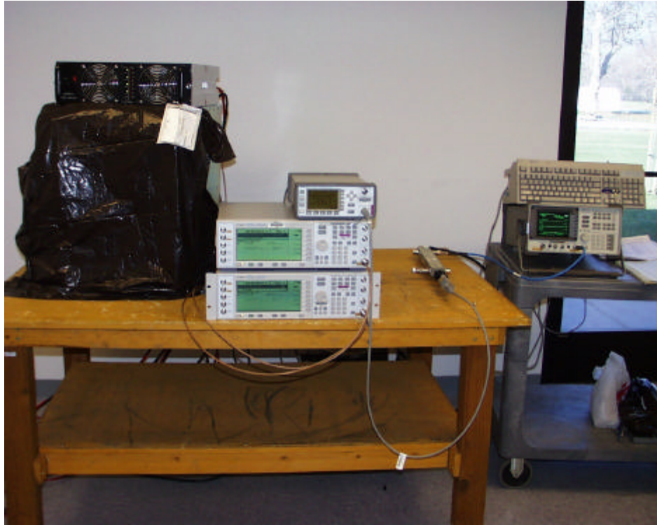
Antenna Terminal Output Measurement Setup
