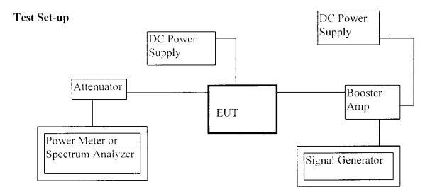
Data on the bandwidth occupied by this transmitter is presented in graphical form using spectrum analyzer plots. Emission bandwidth (per 24.238b, the 26dB BW) was measured with RBW=1 MHz. VBW=1 Mhz..Please refer to Spectrum plots attached.
