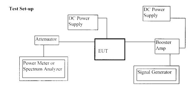
Minimum standard: The magnitude of each spurious and harmonic emission that can be detected when the equipment is operated under conditions specified in the instruction manual and/or alignment procedure, shall not be less than 43+10 log(mean output power in watts) dBc below the mean power output outside a licensee's frequency block.
