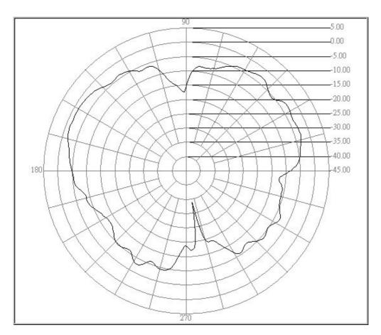
Center freq.(MHz): 2480 Polarization : E Plane
