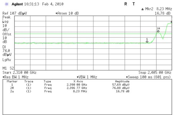
Delta marker at 1% of span = 35.76dB
