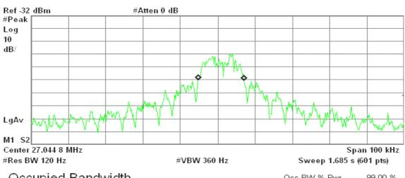
Occupied Bandwidth 12.2513 kHz Occ BW % Pwr 99.00 % x dB -20.00 dB
