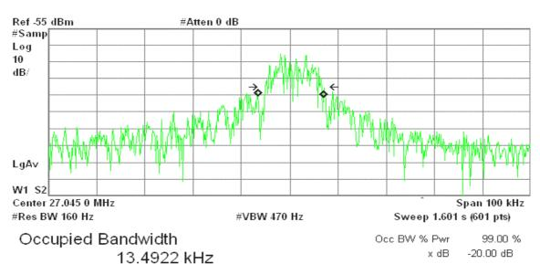
Transmit Freq Error Occupied Bandwidth
