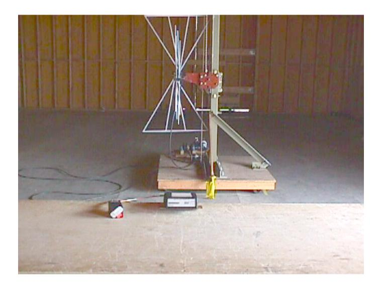
EXHIBIT 9 TEST SETUP PHOTOS RADIATED EMISSIONS AT 3 METERS FCC ID: E5MDS9710-1 PHOTO 1 OF 3
