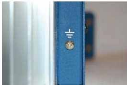
Figure 3-2. Rear Panel Grounding Screw
