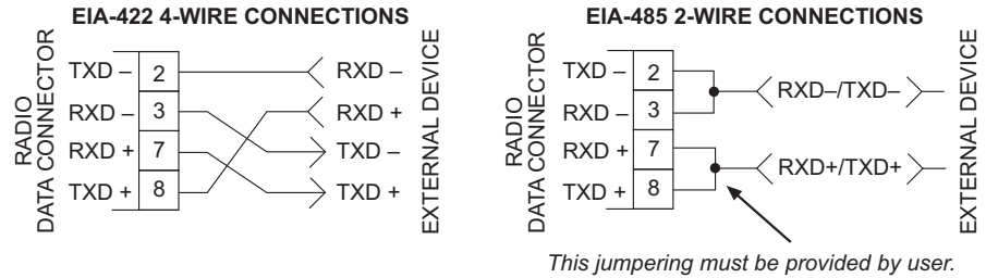
Figure 15. EIA-422/485 Wiring Arrangements
